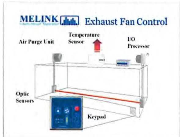
In a Melink system, optical and heat detecting sensors are installed to monitor the cooking activity and automatically adjust the motor speed to as low as 10% based on the amount of heat, steam or smoke present.
